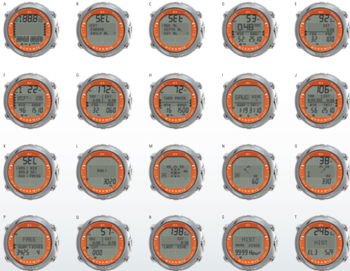
A. Full Segment Display B. Digital Watch Select Function C. Set Mode / Audible Alarms D. Dive / Main E. Dive / Alternate
