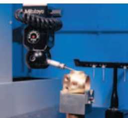
Our precision machine measures every first stage to \pm 0.00002 inch (1/2 micron) to guarantee exceptional performance.
