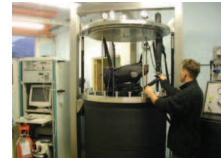
Our ANSTI machine allows us to simulate underwater breathing at extreme temperatures and depths and refine performance.
